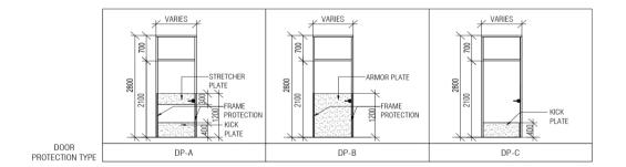
The material is Door Plates Protection - .040" (1.02mm) and .060" (1.52mm) thick Acrovyn or 16 gauge Stainless steel or similar.
