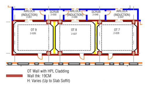
Please refer to the 19cm wall type as shown on Drawing A.11.35 Type 7, see also Drawing A.6.2 reflecting the HPL Cladding location.
