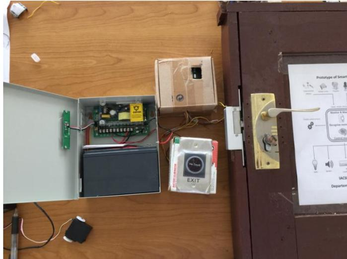
**Figure 3 Overall RFID Tag-based Door Mechanism**
